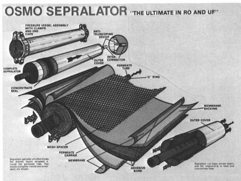
Figure 5. A partially unrolled spiral membrane element known as a sepralator. The sepralator has a permeate tube for collecting the permeate; the membrane is laid onto a permeate carrier material and the edges of the membrane and the permeate carrier are glued together. The membrane is integrally cast onto a backing material as shown in the figure.
